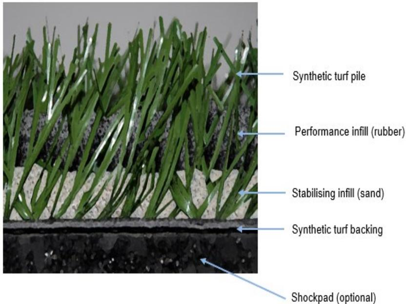
Figure 1 cross section of 3rd generation synthetic turf surface
